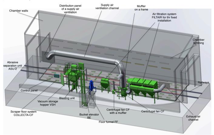
The given technology of metal constructions preparation and protection consists of shot blasting of worked surfaces, followed by the process of collection and regeneration of used abrasive media. Throughout the whole period of this process the certain climatic environment conditions are maintained in the blasting chamber.
