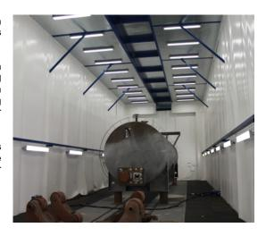
The general view of a blasting chamber with its basic components, based on automatic abrasive collection and regeneration conditions, is presented in the figure below.
